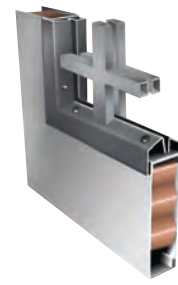
Two-part sandwich-type vision kit with muntins , 18-gauge (0.044”/1.1 mm). Only available non-rated and for 1/4” (6.3 mm) and 1/2” (13 mm) thick glass.
