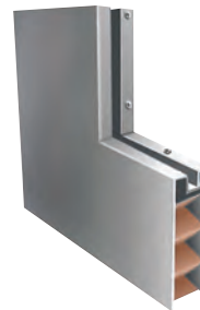
Flush seamless vision kit 16-gauge (0.056”/1.4 mm). Laser welded, available for 1/4” (6.3 mm) to 1” (25.4 mm) thick glass (FKS series).
