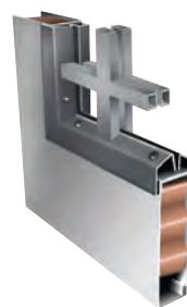
Two-part sandwich-type vision kit with muntins , 18-gauge (0.044”/1.1 mm). Only available non-rated and for 1/4” (6.3 mm) and 1/2” (13 mm) thick glass.
