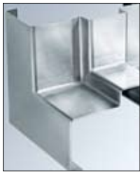
SANITARY WELDED PROFILE Fully continuously welded on exposed side – 5/16" (7.9 mm) seamless radius weld on soffit and rabbets.
